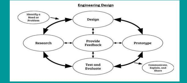
A prototype is constructed based on the design model(s) and used to test the proposed solution. A prototype can be a physical, computer, mathematical, or conceptual instantiation of the model that can be manipulated and tested.
