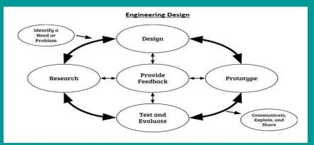
Identify a need or a problem. To begin engineering design, a need or problem must be identified that an attempt can be made to solve, improve and/or fix. This typically includes articulation of criteria and constraints that will define a successful solution.
